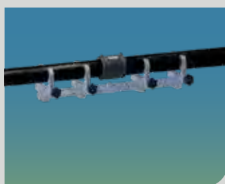
2. Example of clamping and alignment device
